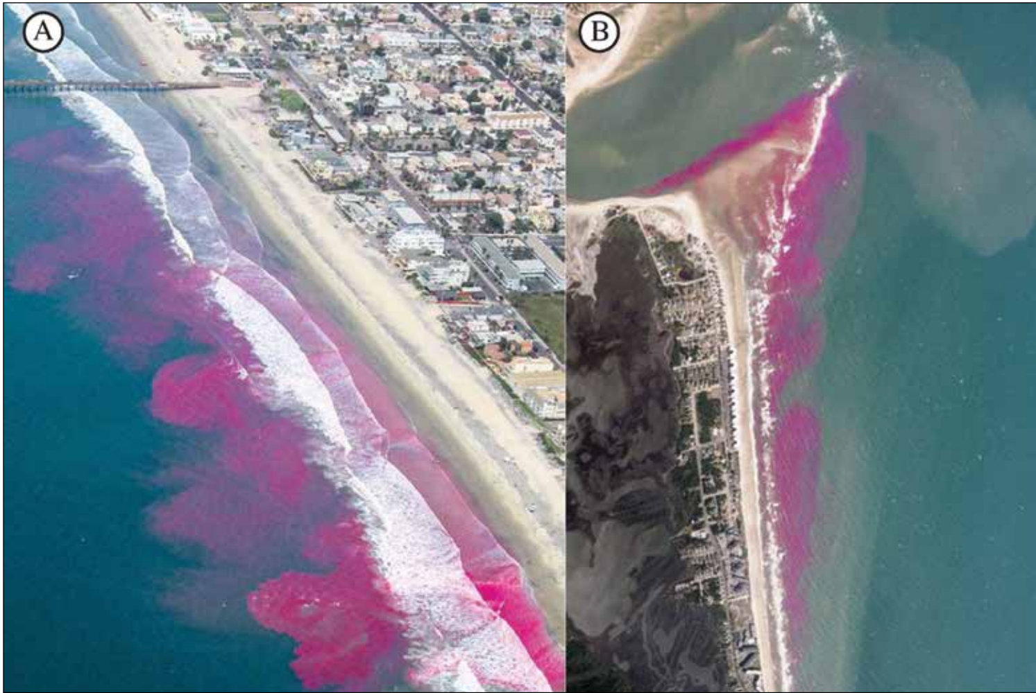
Figure 6: Photographs of non-toxic fluorescent dye tracer (pink water) (A) one hour after continual surfzone dye release at Imperial Beach California (Hally-Rosendahl et al. 2014), and (B) 1.5 hours after continual tidal inlet dye release during ebb tidal flow at New River Inlet, North Carolina. In both cases, dye serves as a mock pollutant and study of its transport and dilution will inform how pollutants from pathogens to chemical contaminants evolve in nearshore waters. (Image from Clark et al. 2014).
