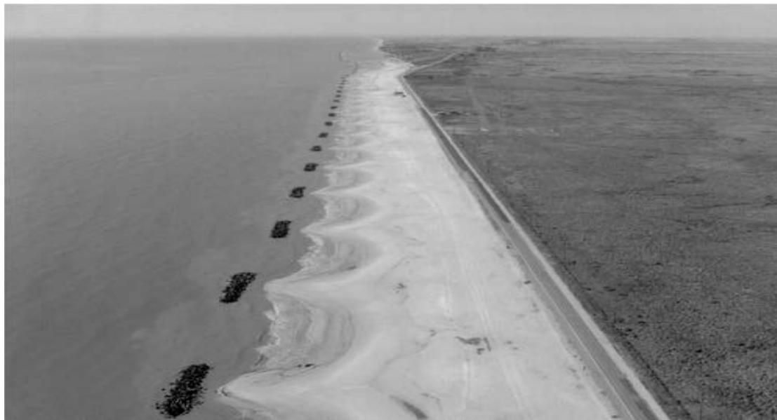
FIGURE 2. Holly Beach breakwater field, looking west from Louisiana towards Texas. The sub-aerial beach in this aerial photograph was constructed using sands buried in an offshore channel located about 3.5 miles offshore. Note the prominent salients forming in the lee of the emergent segmented breakwaters (Mann and Thomson, 2003).
