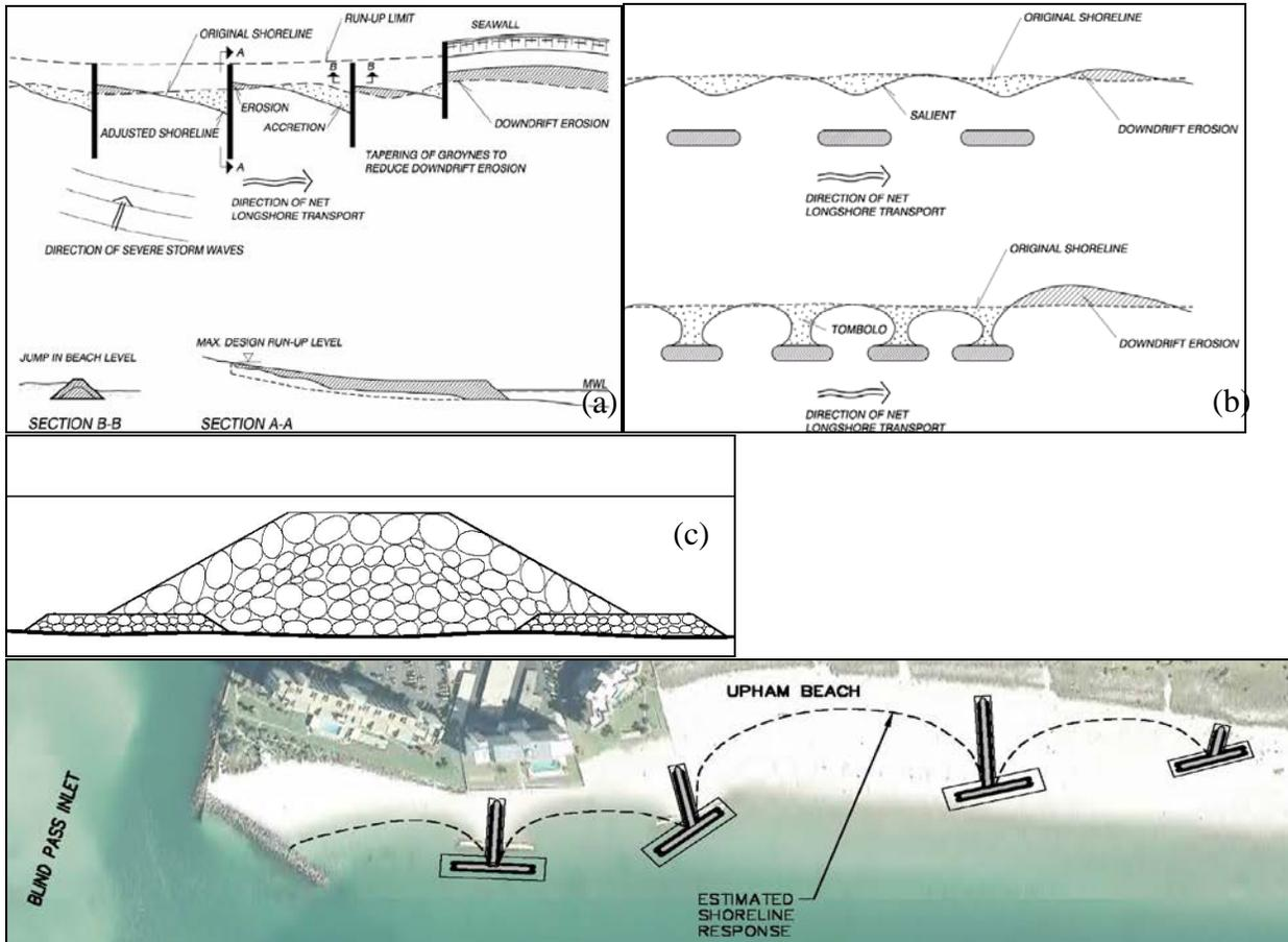
FIGURE 1: (a) Typical beach configuration with groins, (USACE, 2006); (b) Typical beach configuration with detached nearshore breakwaters, (USACE, 2006); (c) Example of a reef breakwater cross-section, (USACE, 2006); (d) Predicted shoreline response for T-head groins at Upham Beach, Florida (CPE, 2010).
